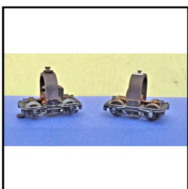
**Ref No:** 1A.21**Category:** Major U.K. manufacturer (believed) mechanism**Description:** Motor bogie, twin-worm-drive, mounted on frame under U-shaped mounting bracket. Believed 20v.ac. Suitable for non-steam outline driving trailer. Qty. 2 Price for pair**Price (£):** 60.00
